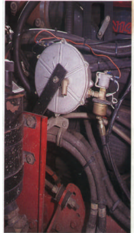
Above: Gas converter mounts on nearside of Cummins N14 Left: Gas is injected (small hoses) into intake pipe before the turbocharger
